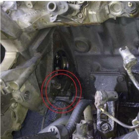
7. INSÉRER LA POMPE 8640A080A (MECANIQUE) ET LA FIXER AVEC LES BOULONS TRAVERSANTS D'ORIGINE, EN PRENANT SOIN DE LA FIXER AU CENTRE DE LA FENTE.
